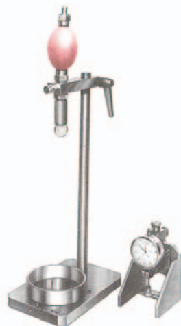
Dropping ball apparatus used in the testing of fresh mortar
