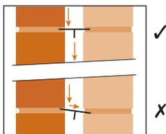
Incorrectly installed wall ties can act as a route for water to pass across the cavity. They should always be bedded horizontal and never slope down towards the inner leaf. Position drips in the middle of the cavity pointing downwards.
