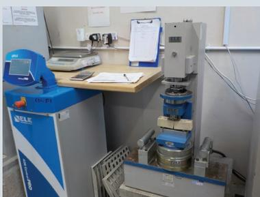
Typical mortar testing facilities
