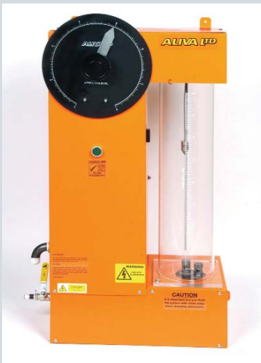
Typical admixture dosing equipment.
