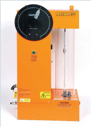
Typical admixture dosing equipment.
