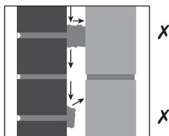
Deposits of mortar on wall ties, large mortar obstructions and mortar extrusions on the inside face of the outer leaf, particularly at bed joints, can deflect or transmit water to the inner leaf. To prevent mortar and debris entering the cavity, use boards or draw battens as the work proceeds.
