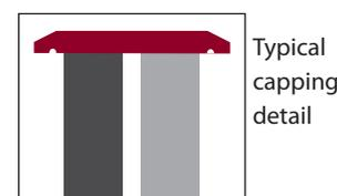
External masonry is much less likely to become saturated if features have been provided to direct run-off water clear of the face of the building. Such features include adequate roof overhangs, projecting throated sills and bell mouths or similar in the case of walls partially clad by tile hanging or other impervious material.
