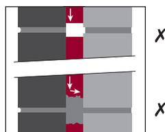
Partially filled cavity using boards, fully filled cavity using boards and fully filled cavity using injected or blown foam or granules are the available insulation systems. They should be correctly installed if problems with rain penetration are to be avoided. Although the materials themselves are waterproof, water can be transmitted across the cavity through voids or gaps in the fill or via mortar extrusions or droppings at joints.
