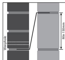
Incorrectly installed cavity trays and DPC's may result in rain penetration problems.
