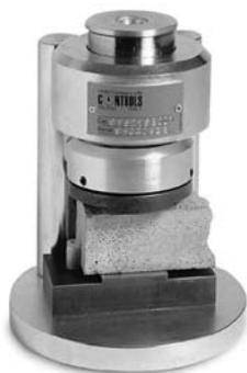
Compressive strength test equipment
