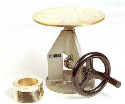
Flow test equipment
