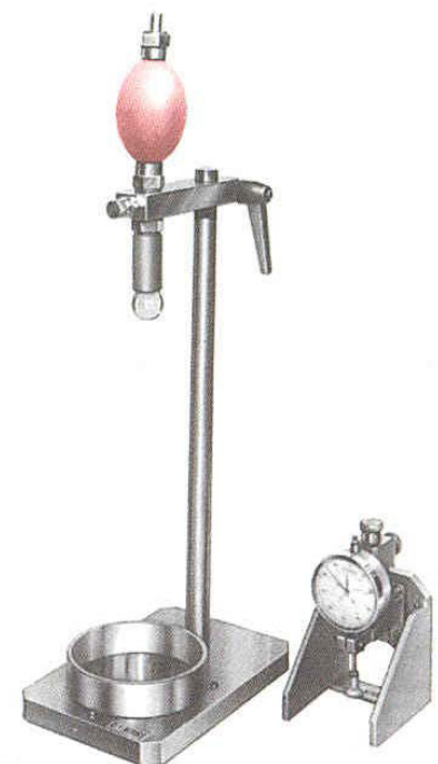
Figure 1: Dropping Ball Apparatus
