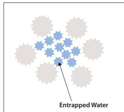
Figure 2: **Flocculating cement particles trapping the mix water**
