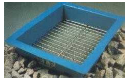
Figure 3: Sieves used for the determination of flakiness index
